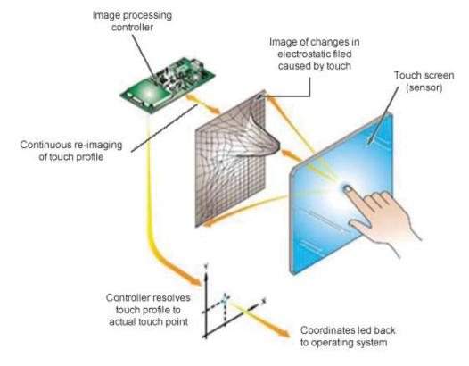
When a conductive object, such as a finger or capacitive stylus, touches the P-Cap touch screen, it distorts the local electrostatic field at that point. This is measurable as a change in capacitance. If a finger bridges the gap between two of the "tracks", the charge field is further interrupted and detected by the controller. The capacitance can be changed and measured at every individual point on the matrix (intersection).
