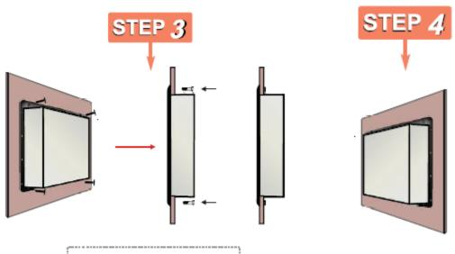
Use M3 screws to drill through the fixture into the mounting holes on the back side of IP65 front bezel
